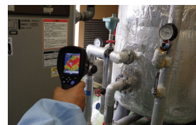
Energy saving diagnostic report in progress Thermography Heat Dissipation Check (Visiting Ohtaya Meat Co., Ltd.)
