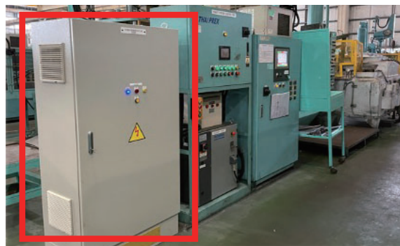
The equipment was installed between the control panel of the casting machine and the hydraulic pump motor.
